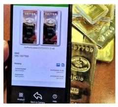
FeaturePrint® is an optical AI technology that digitises items to create a one-of-akind unique identifier that, again, does not involve any marking, modification or addition to the product. Using a camera, FeaturePrint enables identification, authentication, and traceability of individual items out of millions of similar ones.
