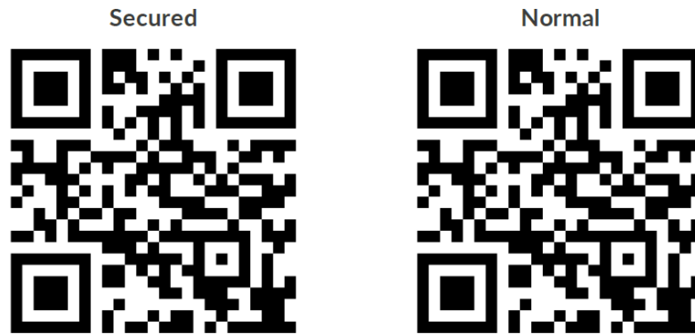
Figure 2: Secured and Normal QR code cannot be distinguished with the naked eye
