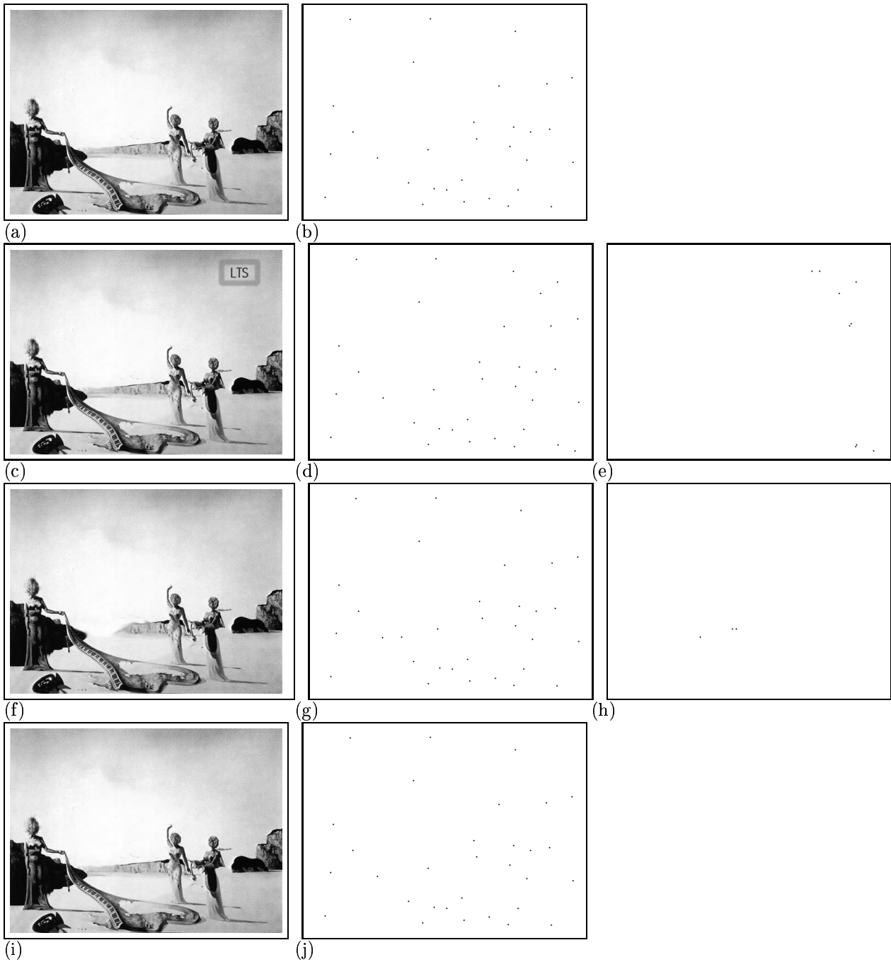
Figure 1: Authentication of “Piano” image: (a) original image; (b) feature-points of (a); (c) original image modified on the top right corner; (d) feature-points of (c); (e) difference between (d) and (b); (f) original image edited to remove image features near the center of the image; (g) feature points of (f); (h) difference between (g) and (b); (i) JPEG compressed/decompressed version of (a) with 80% quality; (j) feature-points of (i). Note that the points in (e) and (h) correspond to only the image-regions modified in (c) and (f) respectively. The points in (j) are within 1 pixel of the corresponding points in (b).
