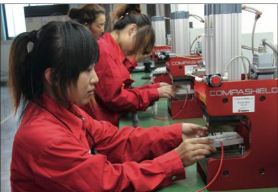
The gaskets are adapted for customers by splicing to the right length.
