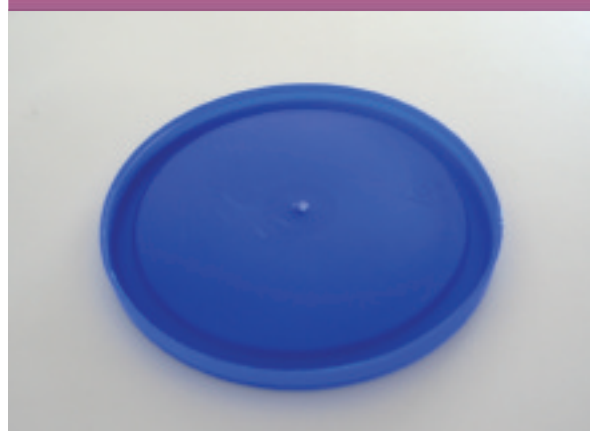
Figure 4: Plastic closure of a jar of baby food which can be identified with a reference template of the mould used to produce it
