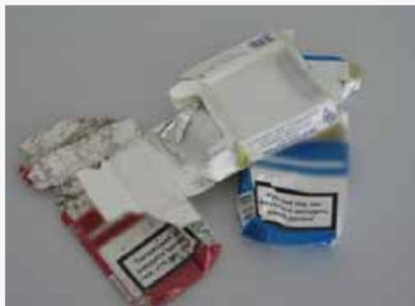
The Cryptoglyph® invisible marking, based on micro differences of thickness within the varnish layer, applied with regular rotogravure printing equipment, showed outstanding properties of robustness in used packaging which had been discarded in the litter. This rubbish, even when folded, soiled and partly torn up, still contained enough invisible information to enable a highly reliable “Genuine or Fake” verdict.
