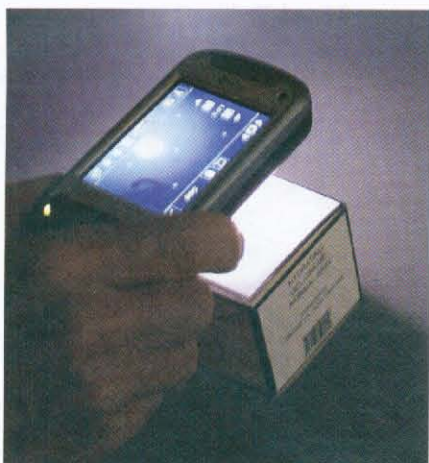
Remote authentication of Cryptoglyph-protected packaging, using a standard PDA camera/phone.
