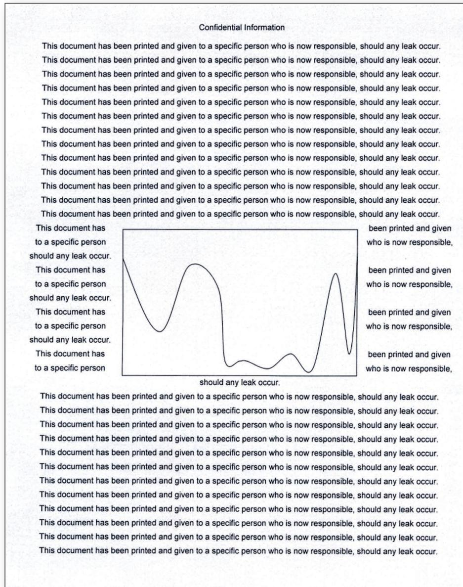
**Figure 4. Word-processing printout from a 1200-dpi black-and-white laser printer. Photocopy-resistant information ciphered in visible gray dots**
